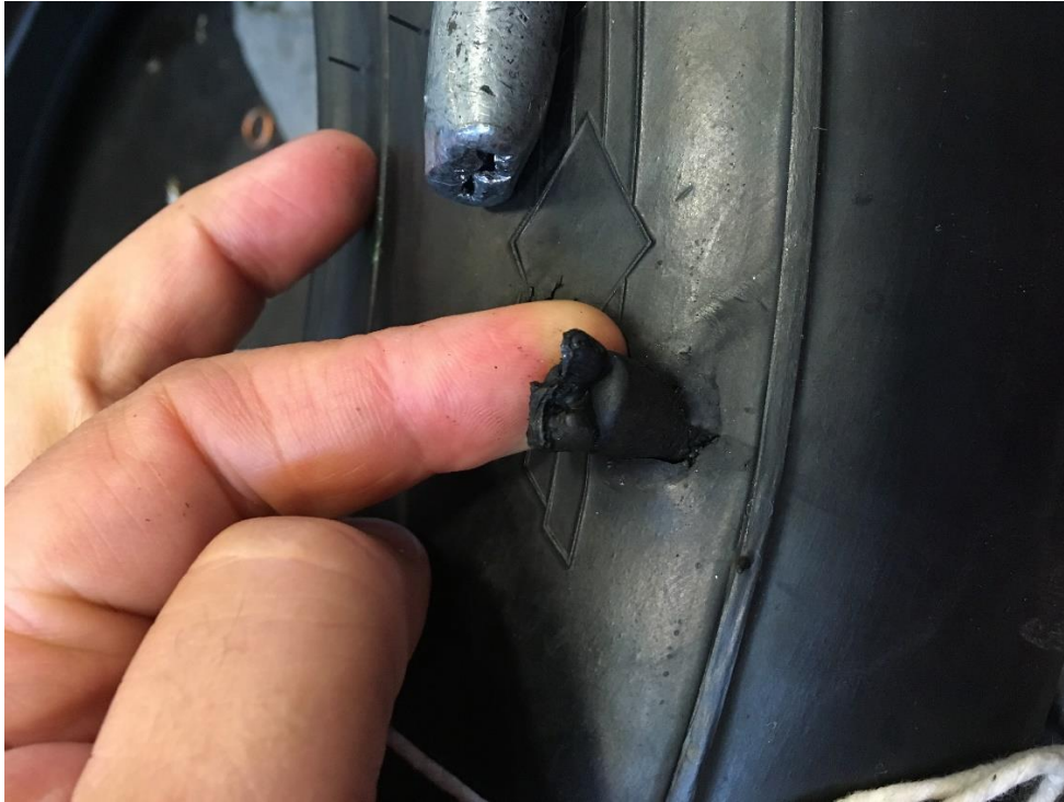
Fig 3: Indications metal was molded into tire
