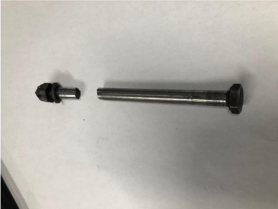
Pic 2: Sheared bolt
